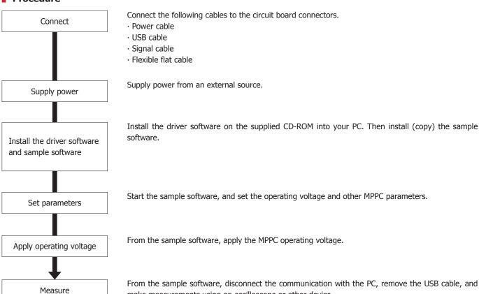
make measurements using an oscilloscope or other device.
